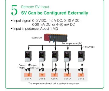
Synchronous temperature-rise control is available in combination with 2-degrees-of-freedom PID.
