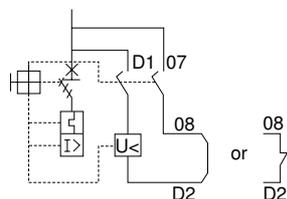
In addition to the functions of the undervoltage trip device, this device completely opens the main circuit and control circuit when the MMS is turned OFF. However, when the MMS is tripped by a drop in the control circuit voltage, it must be reset.
