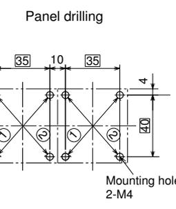
Use the two mounting holes on a diagonal line ① or ② to mount a contactor.
