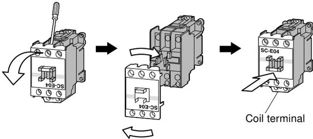
**For SC-E1 to SC-E3 magnetic contactors**
