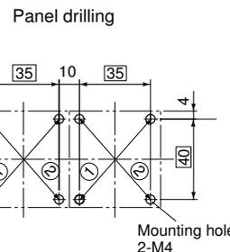
Use the two mounting holes on a diagonal line ① or ② to mount a contactor.
