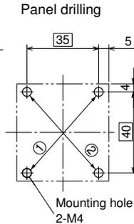
Use the two mounting holes on a diagonal line ① or ② to mount a contactor.
