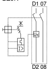
There may be no trip indication and no opening of the auxiliary contact even though the MMS is tripped due to short-circuit, overcurrent, or phase-loss.
