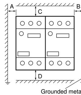
When frames are mounted side-by-side, operating conditions such as a high ambient temperature or using the maximum setting for continuous carrying current may cause slight changes in operating characteristics due to temperature rises. Under such conditions, it is recommended that the frames be separated by at least 5mm.
