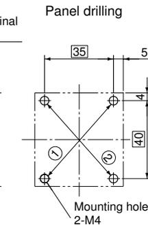
Use the two mounting holes on a diagonal line ① or ② to mount a contactor.
