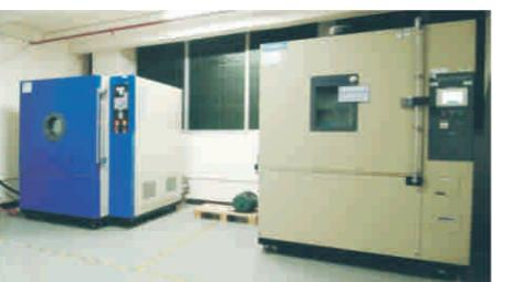
Low Pressure Test Chamber (L)
